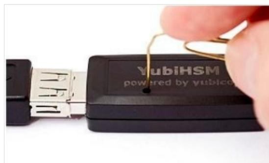
Keep the switch pushed while inserting the device into the host USB port and hold it activated until the LED by the switch starts to
