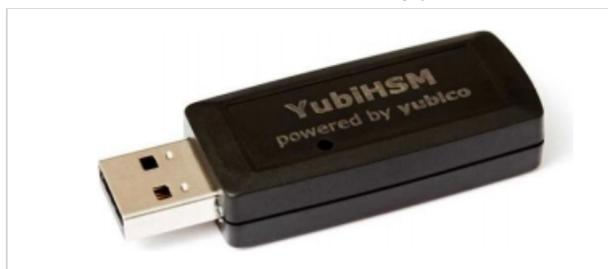
No low-level drivers are needed as the YubiHSM implements the USB-CDC serial communication class. The YubiHSM is intended to operate in conjunction with a host application (WebADM in our case).
