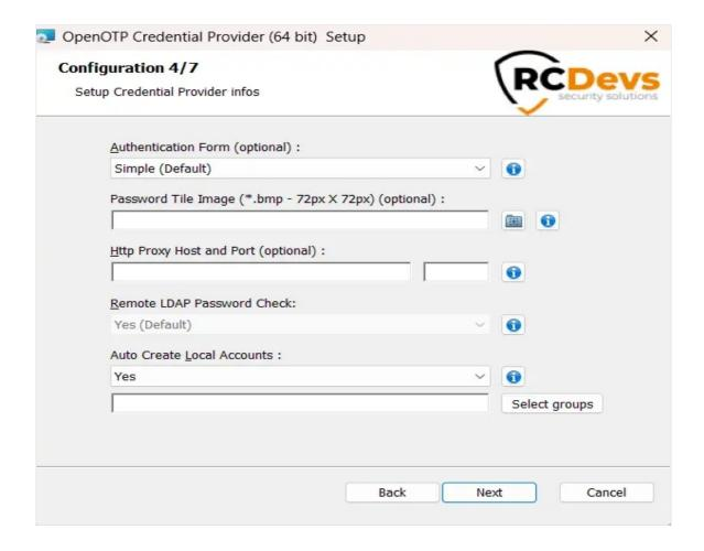
That means, the LDAP password will not be sent to OpenOTP and will only be checked locally by the Windows machine. In the registry, the key related to this setting is check\_ldap. This key is set to 0 to send the -LDAP flag to OpenOTP, which tells it to not check it. When 1 is set, the user password provided during the authentication will be sent by the Credential Provider to OpenOTP and checked there.
